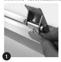
Secure angle bracket with hex key. Mark and drill holes for screws.
